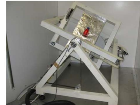
Random Positioning Machine (Laboratory Marcel Egli, ETH Zurich)
